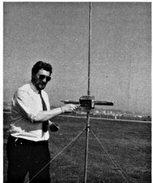
Fig. 2.7: The completed ringbase with radiating element fitted and mounted on mast.
